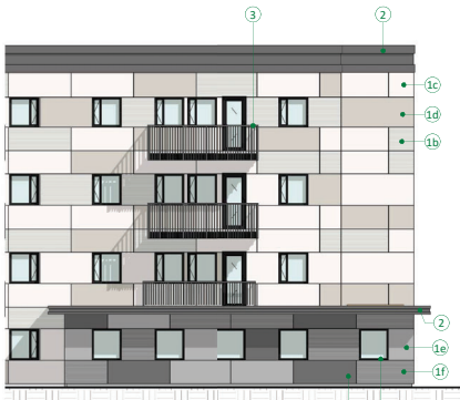
1 BUILDING A - PARTIAL SOUTH ELEVATION 1 : 100
