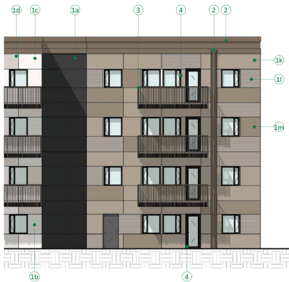
2 BUILDING C - PARTIAL EAST ELEVATION 1 : 100
