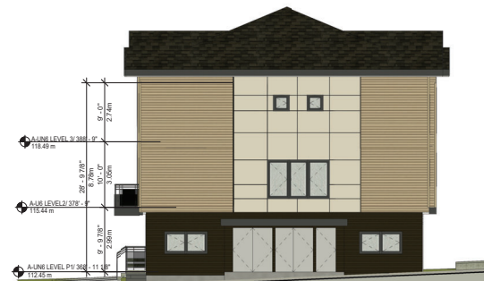
④ Elevation BLD A - West 1/8" = 1'-0"
