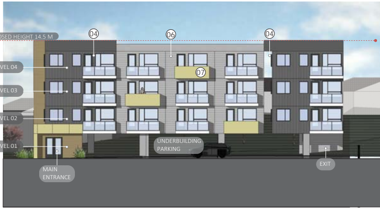
FRONT ELEVATION | BUILDING B | Scale 3/32" = 1' |
