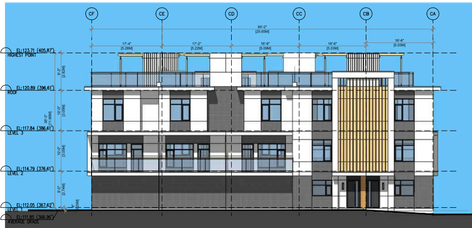
BLDG C EAST ELEVATION
