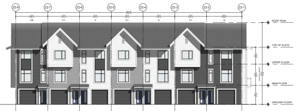
4 BUILDING 22 WEST ELEVATION 1:100
