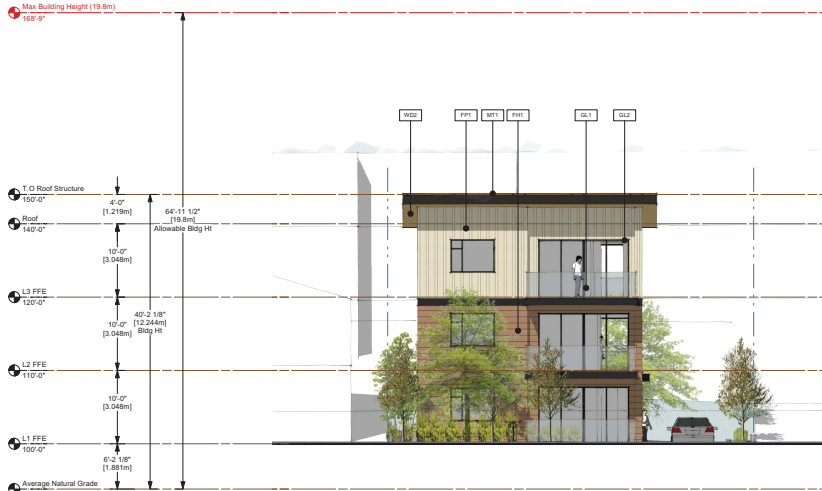
3 South Elevation (Facing Bradley Street)
