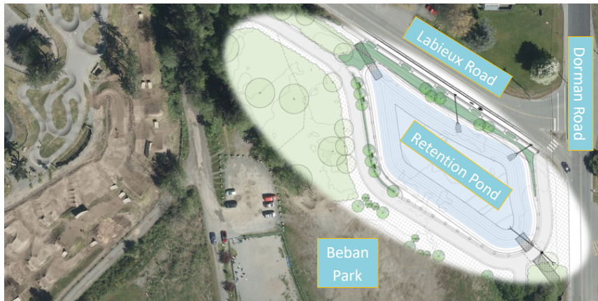
New Stormwater Retention Pond
