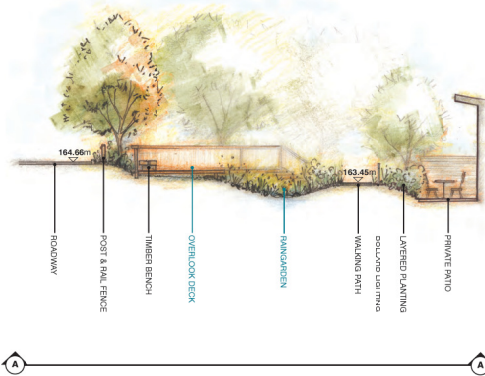
A SECTION / ELEVATION SCALE 1:100 CENTRAL RAINGARDEN
