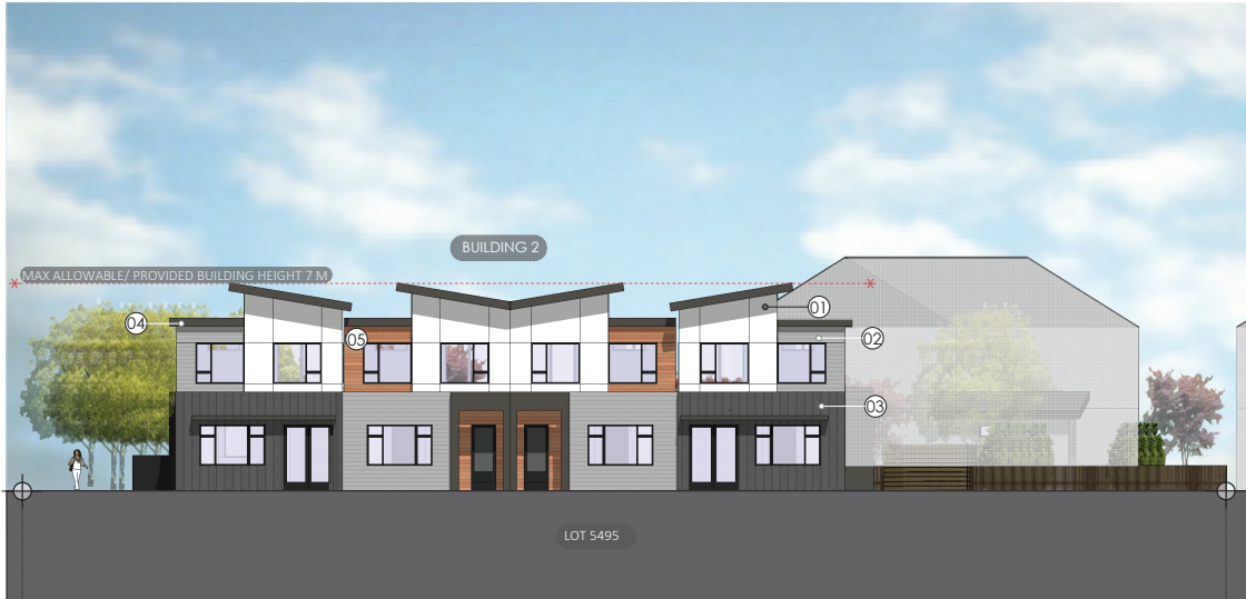
SOUTH ELEVATION | TOWNHOMES | BUILDING 2 FRONT ELEVATION | Scale 1/8" = 1' |
