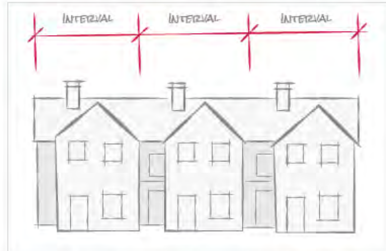
Breaking up a building's facade into a series of intervals creates a more pleasing human scale expression.
