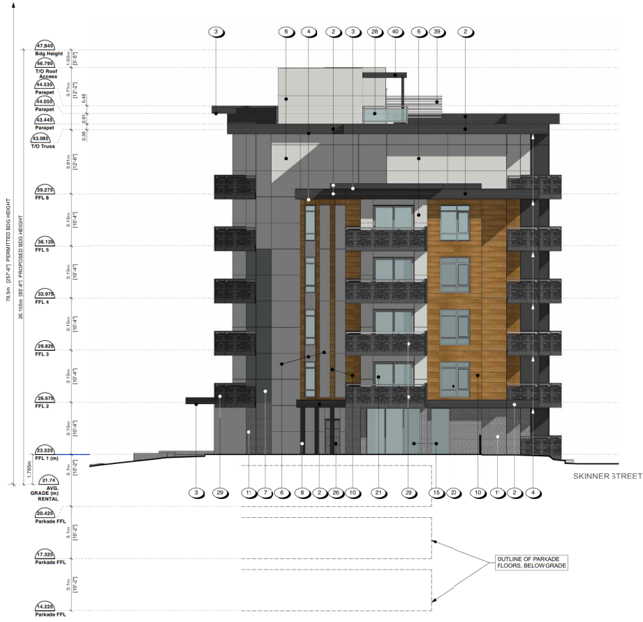
1 Rental Building - North Elevation Scale: 1/8" = 1'-0"
