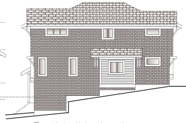
2 Right Side Elevation 3-A200 Scale: 3/16" = 1'-0"
