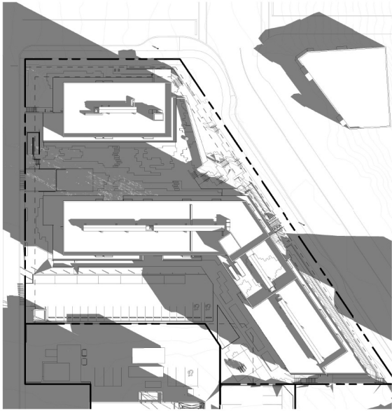
1 | SITE PLAN - SPRING EQUINOX/MARCH 19 - 9 AM SCALE: 1:500
