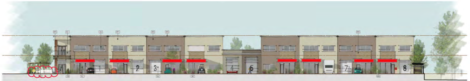
1 NORTH ELEVATION - BLDG B Scale 3/32" = 1'-0"
