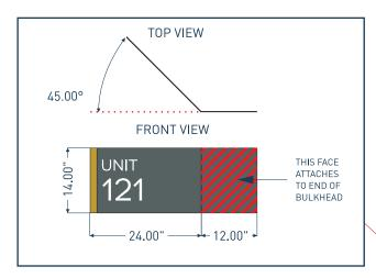
CONSTRUCTED FROM BENT 1/8" ALUMINUM, PAINTED TO MATCH BULKHEAD, WHITE A9 VINYL TEXT,
