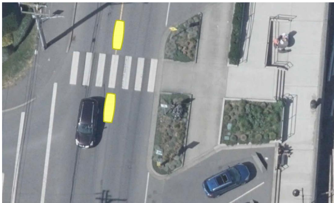
Figure 3. Layout of Crosswalk with Traffic Calming Curbs
