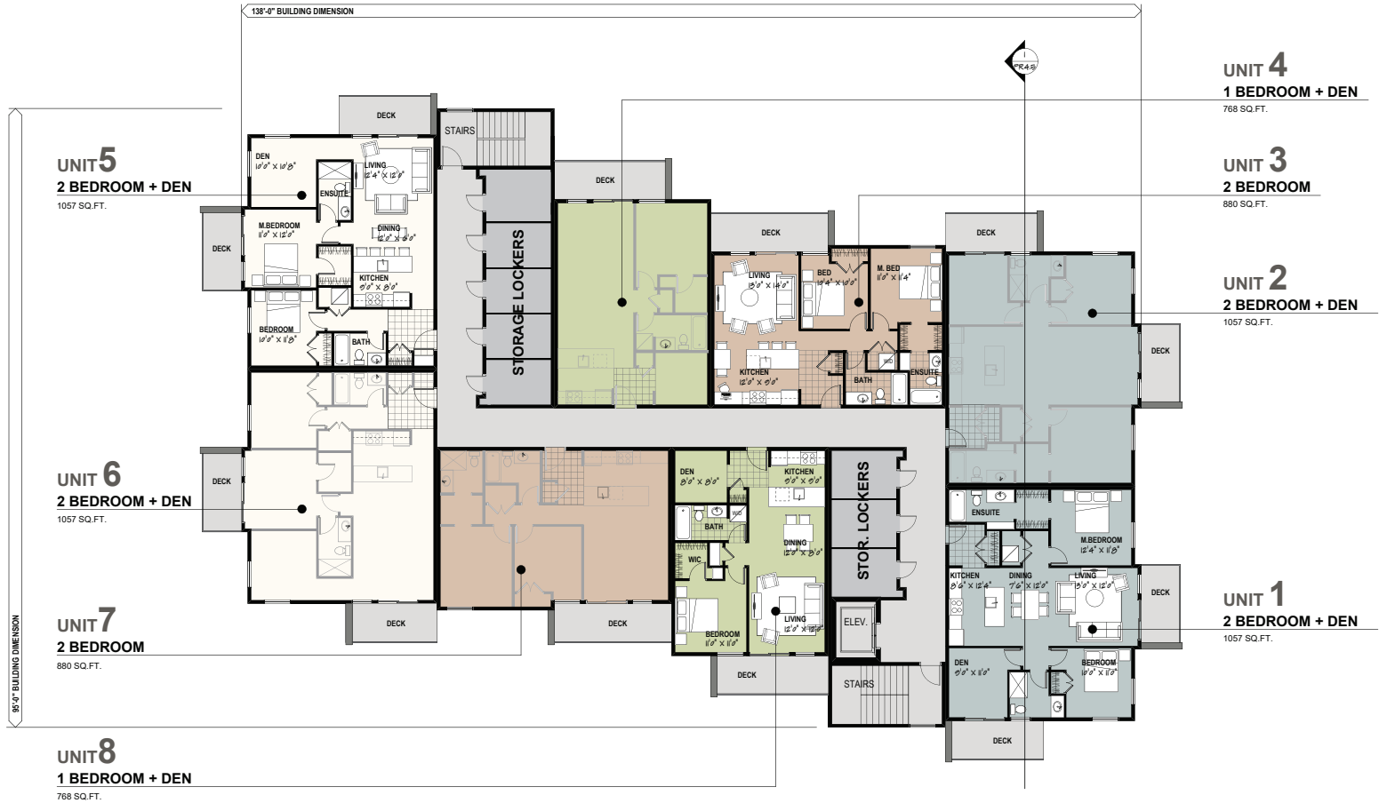
TYPICAL FLOOR PLAN - LEVELS 2,3,4,5 8 UNITS / FLOOR 9,598 SQ.FT. PER FLOOR
