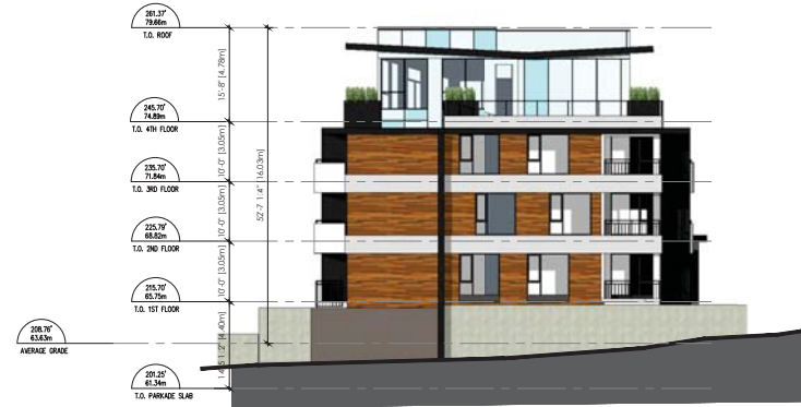
2 17109 - BUILDING D WEST ELEVATION 3/32"=1'-0"
