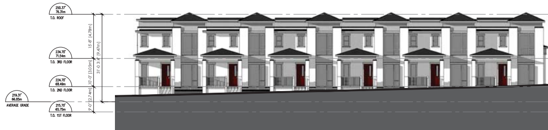
5 17109 - BUILDING B SOUTH ELEVATION 3/32"=1'-0"
