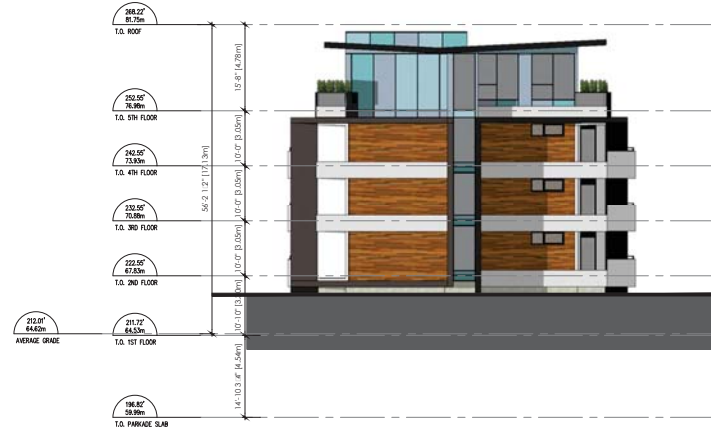
2 17109 - BUILDING F SOUTH ELEVATION 3/32"=1'-0"
