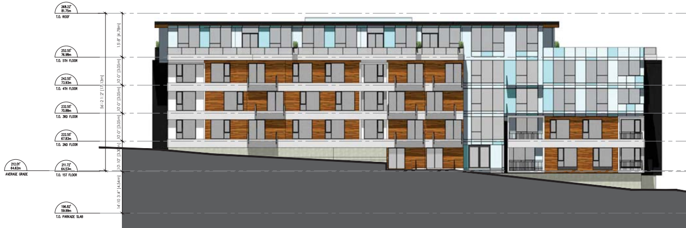
3 17109 - BUILDING F EAST ELEVATION 3/32"=1'-0"
