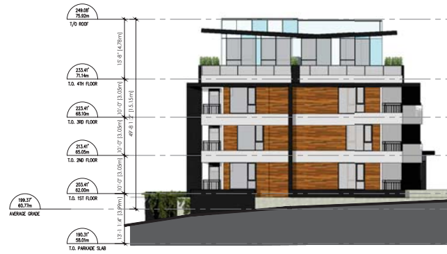
2 17109 - BUILDING E WEST ELEVATION 3/32"=1'-0"
