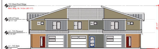
3 Front Roof Type 1 Front Elevation - A3 3/32" = 1'-0"
