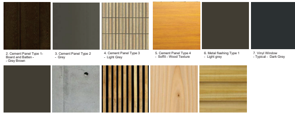
1. Metal Guardrail - Light Grey 2. Cement Panel Type 1 - Board and Batten - Grey Brown 3. Cement Panel Type 2 - Grey 4. Cement Panel Type 3 - Light Grey 5. Cement Panel Type 4 - Soft - Wood Texture 6. Metal Flashing Type 1 - Light grey 7. Vinyl Window - Typical - Dark Grey 8. Metal Guardrail - Light Grey 9. Exposed Concrete 10. Aluminum Battens with wood texture 11. Heavy Timber column and beam 12. Cedar Fence 13. Cedar Fence
