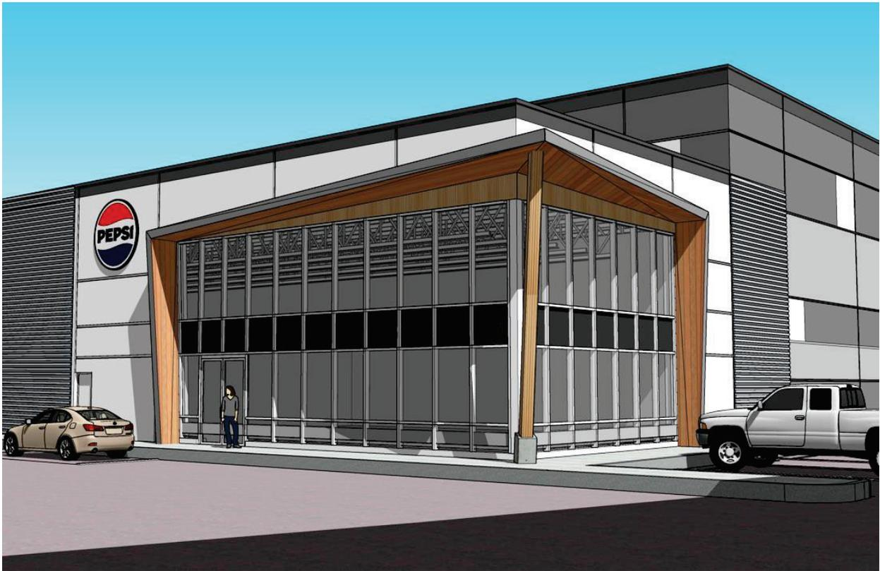
A series of windows along the fleet shop provides visual relief to the solid concrete walls. Additionally, playful patterns created with corrugated metal panels and elastomeric paint on the tilt-up walls add visual interest and break the monotony of the long façades.
