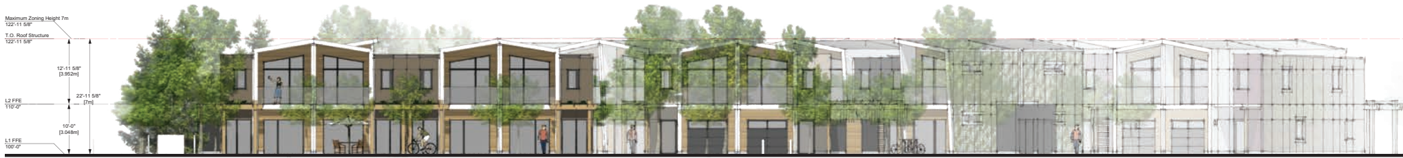
4 South Elevation (Bird Sanctuary Drive) Scale: 1/8" = 1'-0"
