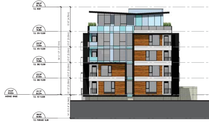
2 17109 - BUILDING F NORTH ELEVATION 3/32"=1'-0"
