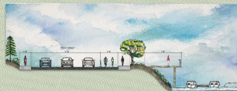
7m boardwalk in Boat Basin is an extension of the existing cantilevered boardwalk 3m bi-directional on-road cycle track on Front St. to be accommodated by reducing traffic lanes
