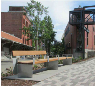
BANCAL BENCH Materials: Ash or IPE wood, steel frame (powdercoated) Mount: Surface mounted Supplier: landscapiforms
