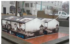
moving the cannons, a solution to cover the cannons and leave them on site was implemented. The covers are made out of aluminum and needed to be covered or painted. Opting to cover them with a heavy duty vinyl wrap with an anti graffiti coating was a more cost effective and maintenance friendly solution and potentially creates an opportunity to share some historical images and perhaps highlight some of the museum's initiatives.
